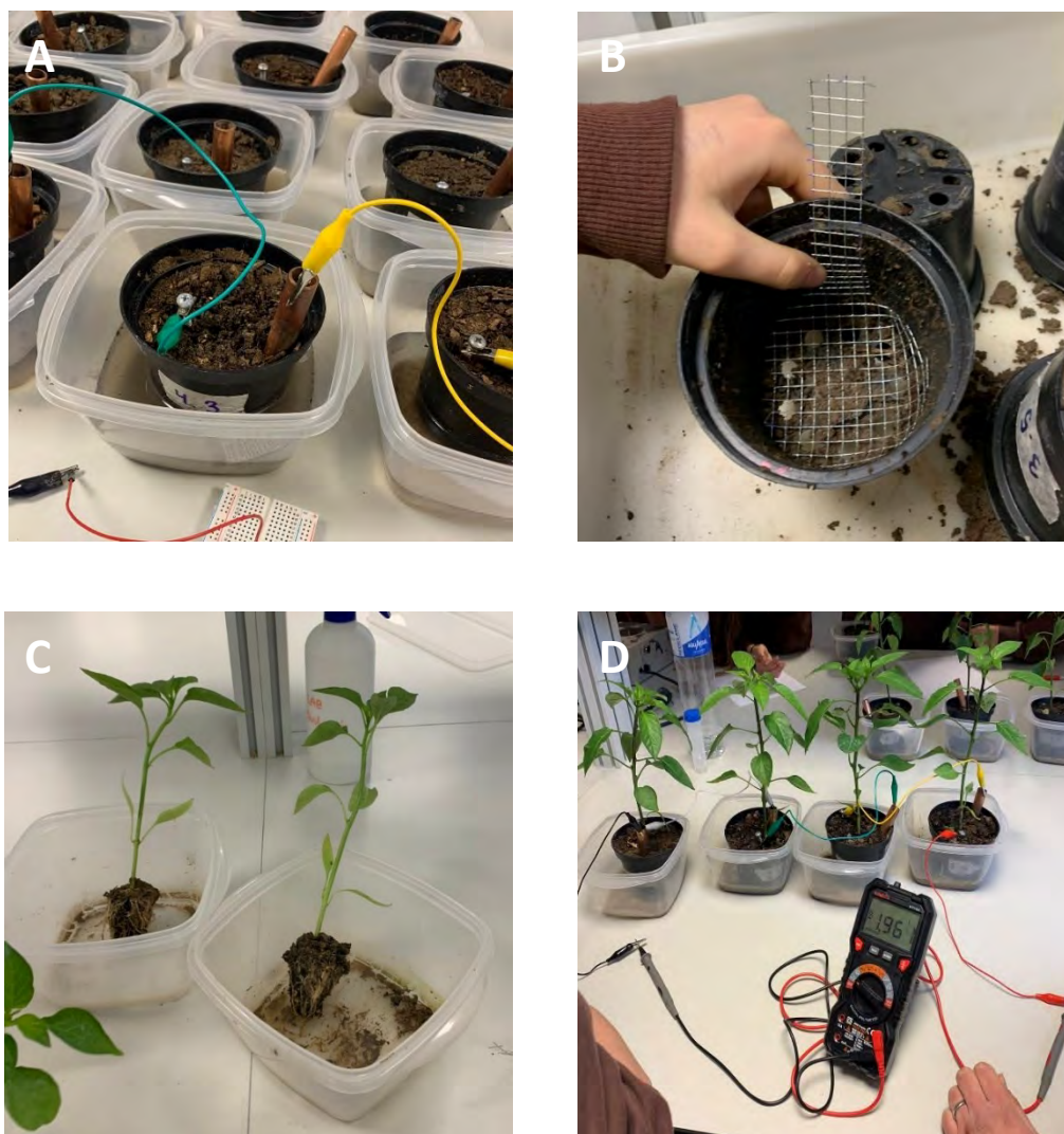
Figure 1. An overview of the experimental setup: Electrodes A, made of a metal mesh and copper foils (A); Electrodes B, made of galvanized screws and copper tubes (B); pepper plants before transplanting (C) and electrical voltage and intensity measurement with a professional digital multimeter by connecting pots as a series circuit (D).
