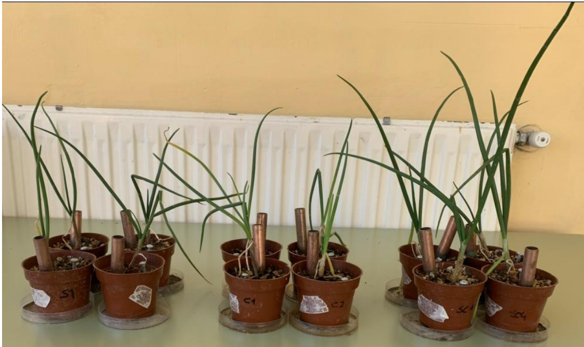
Figure 1. Pots used in this experiment: S (soil), C (compost) and SC (soil and compost at 50%). In each pot, a copper tube and galvanized screws were used as a cathode and anode, respectively.
