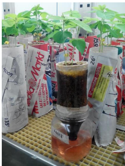
Figure 1. Leonard Jar system used in this study.
