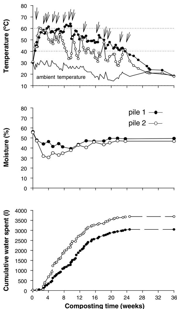
Fig. 1. Temperature profile (arrows indicate turnings), moisture content and water added during composting (pile 1: mechanical turning and pile 2: forced ventilation combined with mechanical turning).
