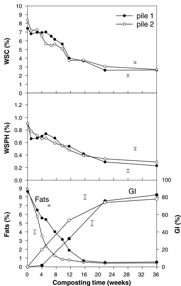
Fig. 4. Changes in water-soluble organic carbon (WSC), water-soluble phenols (WSPH), fat content and germination index (GI) during composting (pile 1: mechanical turning and pile 2: forced ventilation combined with mechanical turning). The bars correspond to the least significant difference at  $P < 0.05$ .
