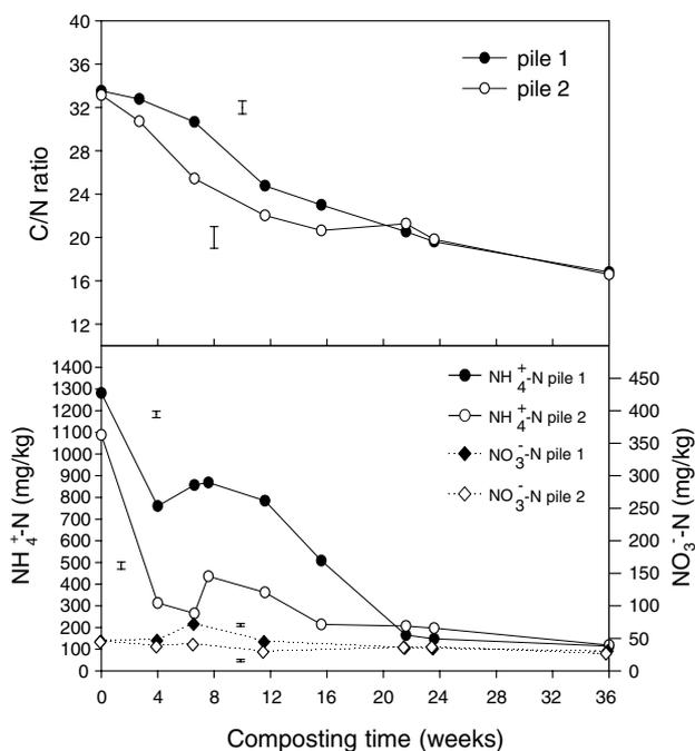
Fig. 3. Evolution of the C/N ratio and inorganic nitrogen ( $\text{NH}_4^+\text{-N}$  and  $\text{NO}_3^-\text{-N}$ ) during composting (pile 1: mechanical turning and pile 2: forced ventilation combined with mechanical turning). The bars correspond to the least significant difference at  $P < 0.05$ .
